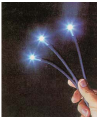
Fibre optic lighting has virtually no heat, no ultra violet light, and is very energy efficient. Only light and not electricity is transmitted through the fibres, so is safe to use near water
